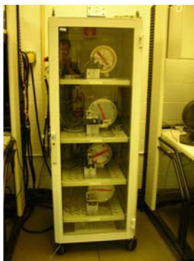
Figure 3. The tone ring tower used to generate wheel speed sensor signals.
