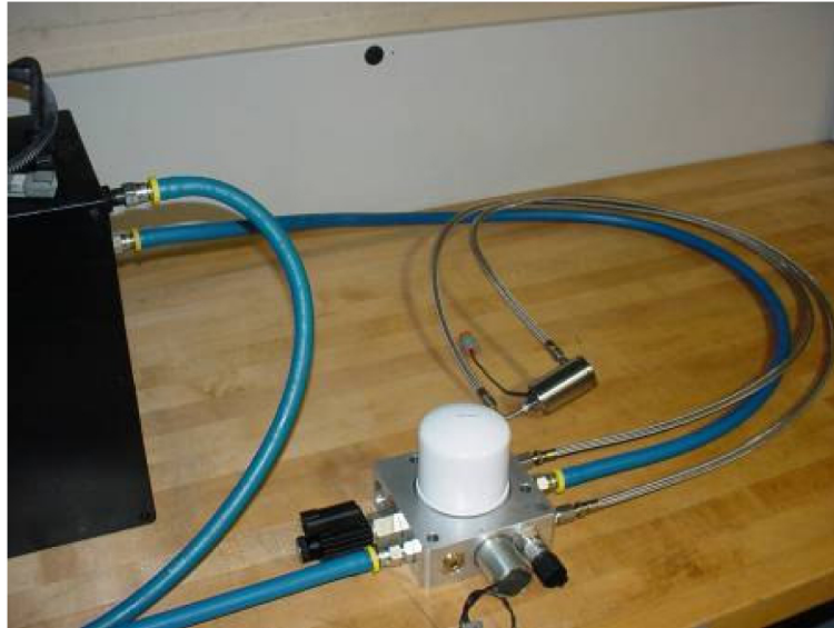
Figure 7. FSA components; auxiliary fuel pump housing, fuel manifold assembly, injector, and associated fuel lines.
