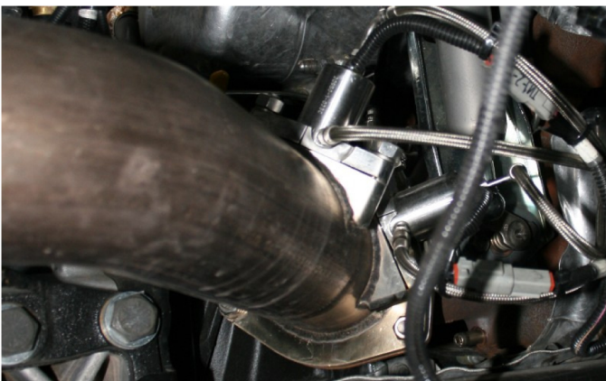
Figure 6. Aftertreatment fuel dosing system mounted to the vehicle exhaust pipe
