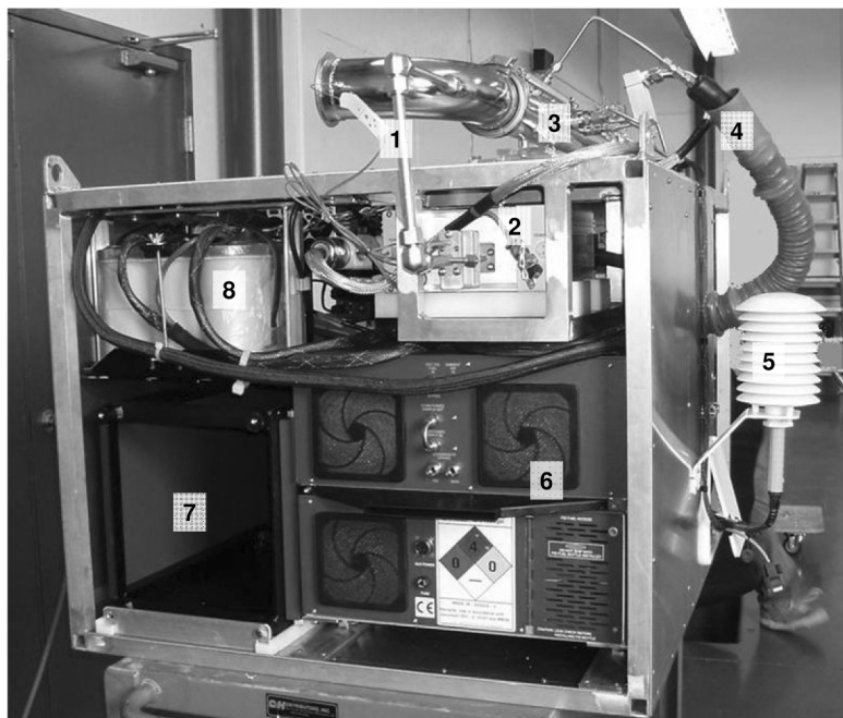
Figure 1. Sampling enclosure with instruments : (1.) SEMTECH MPS sample line, (2.) SEMTECH MPS, (3.) exhaust flowmeter, (4.) heated gaseous sample line, (5.) ambient humidity and temperature sensors, (6.) SEMTECH DS, (7.) space for SEMTECH filter box (not installed), and (8.) batteries for backup power.
