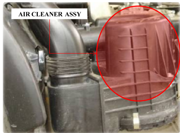
Figure 1.0. (a) Resonator on Clean Side piping of AIS (b) Air cleaner Assembly with Extended Air Cleaner Volume
