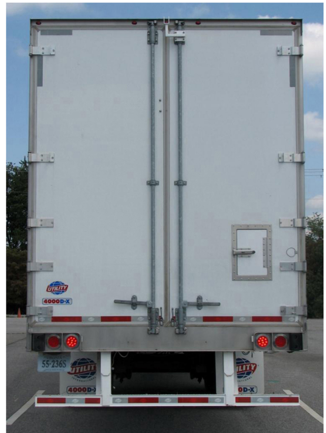
Figure 1. Two LED-unit Steady Brake Light Configuration (Baseline Condition)
