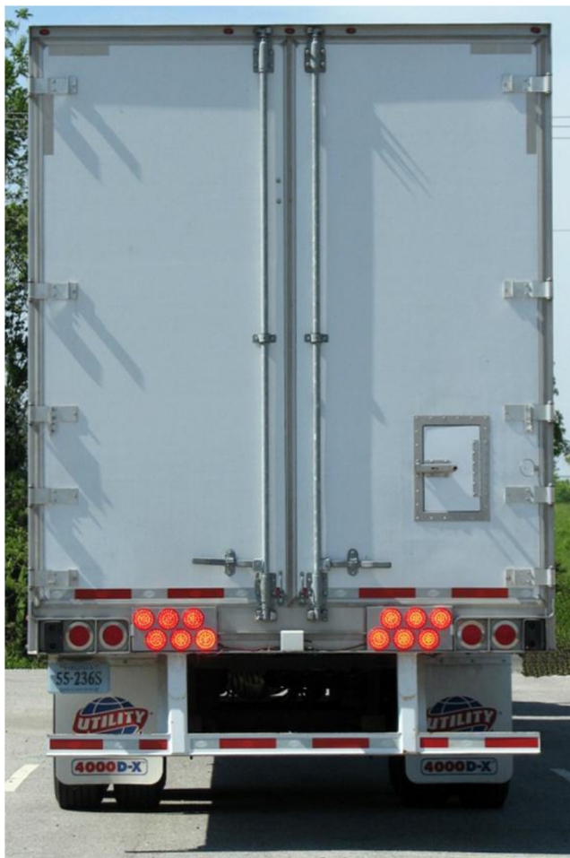
Figure 2. Twelve High-output LED-unit Ganged Main Bumper Configuration
