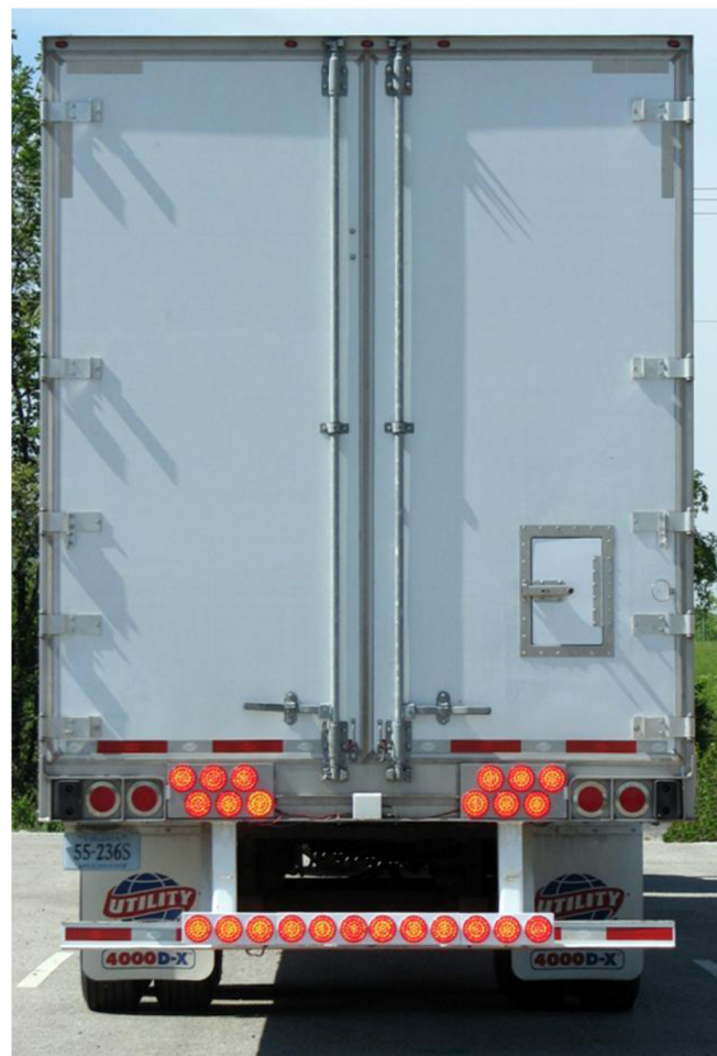
Figure 3. Twelve High-output LED Units Ganged and Positioned on Main Bumper Combined with Twelve High-output LED Units on ICC Bumper
