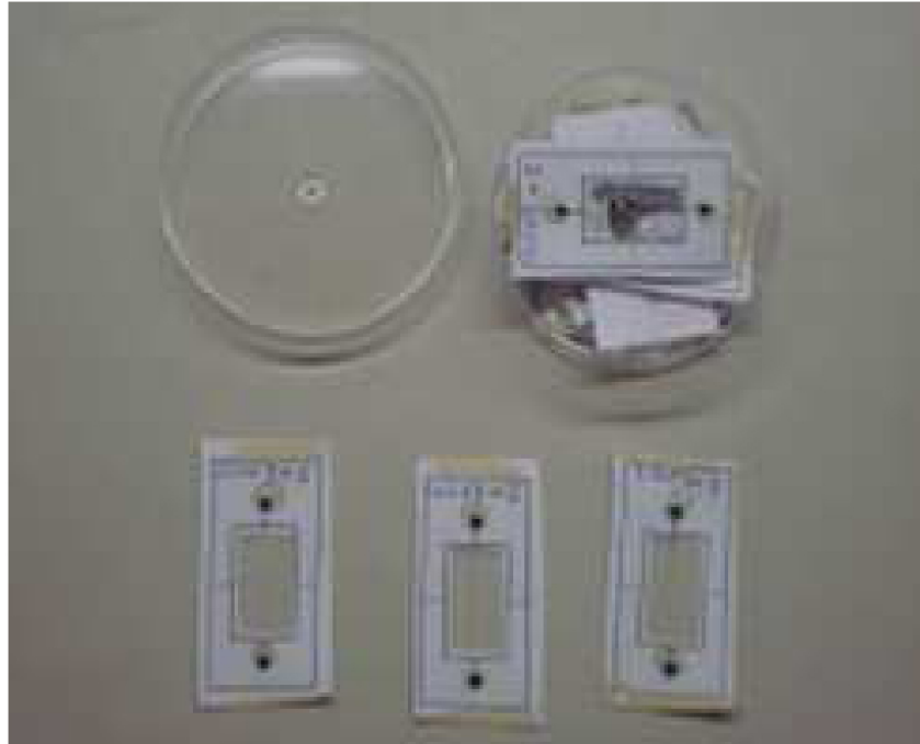
Figure 2. Prepared samples for measuring tensile strength of flax fiber
