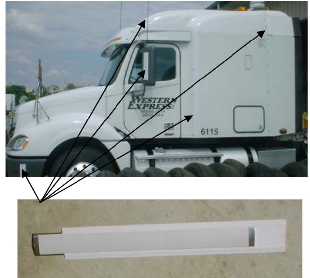
Fig 1. Deturbulator Strip (Bottom) and installation on Flatbed Tractor (Top)
