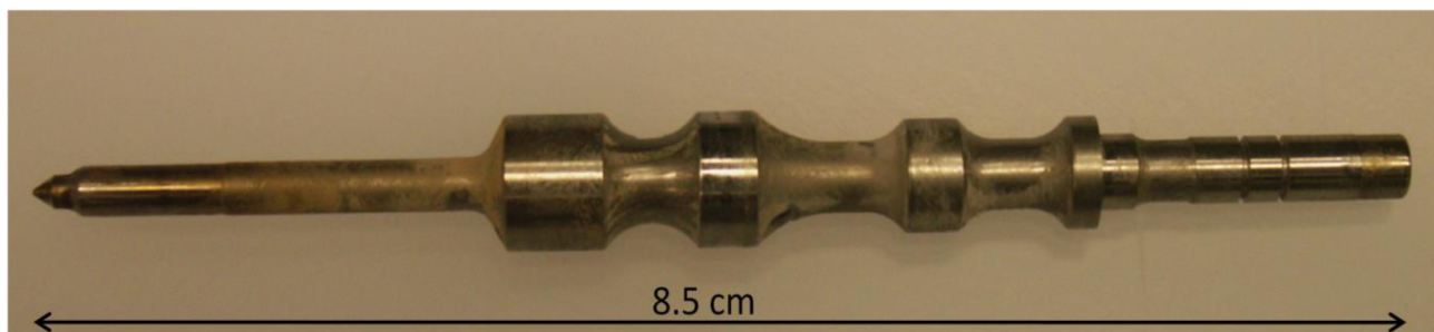
Figure 1. Needle taken from an UPCR injector that showed symptoms of sticking.
