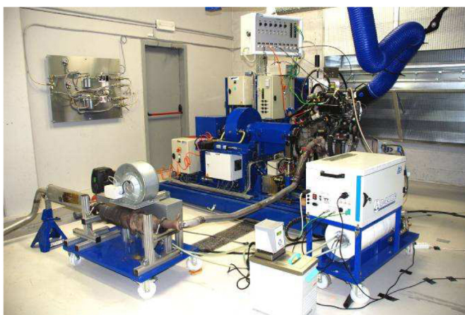
Fig. 2. Engine installed on test bed with oil consumption measurement in the exhaust line (front left) and fuel dilution monitoring device (front right)
