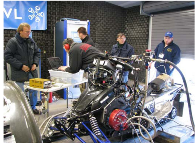
Figure 1. Stationary snowmobile emissions testing at the 2009 SAE CSC
