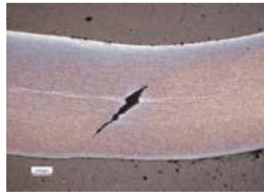
Figure 2. AHSS cracking initiates from the central segregation (from Reche and Sturel, 2009)
