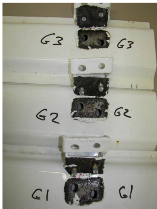
Figure 5. Expandable Sealer with Wire Mesh Samples at End-of-Test
