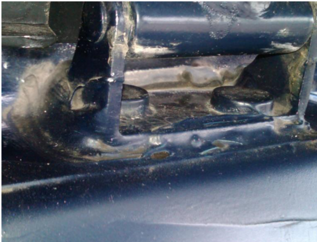
Figure 3. Liftgate hinge shown with paint shop applied sealer around the perimeter of the hinge.
