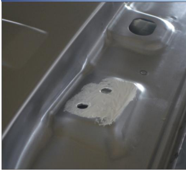
Figure 2. Roof panel shown with roll-on sealer applied prior to liftgate hinge installation.
