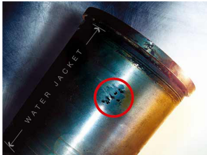
Figure (1-a). Pitting in the cylinder liner.
