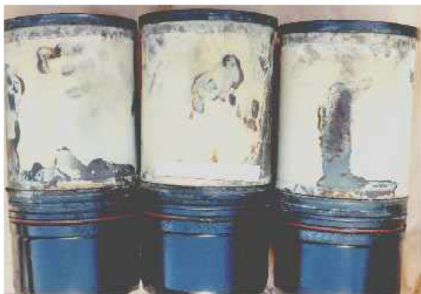
Figure (1-b). Thick layer of scale formation.
