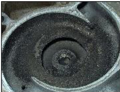
Figure (1-c). Corrosion of engine's water pump.
