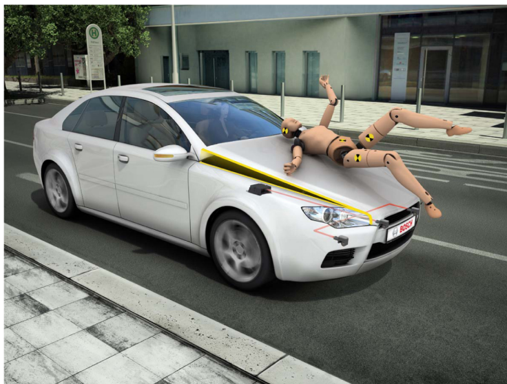
Figure 1. An electronic pedestrian protection system using three accelerometers mounted in the bumper fascia
