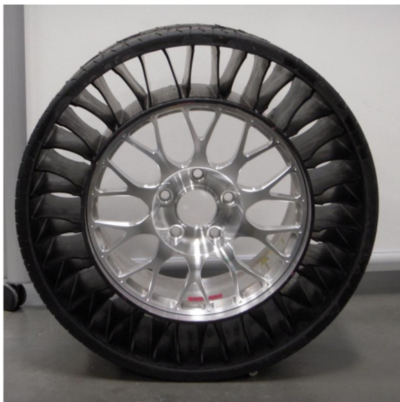
Figure 2. Prototype Tweel tire used for testing at Clemson University and Michelin.
