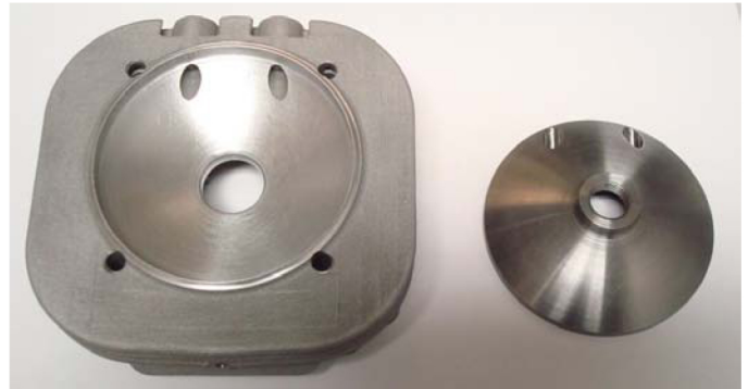
Figure 2. Cast Aluminum Head and Steel Insert
