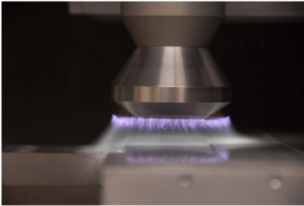
Figure 2. Openair® plasma during the treatment of a polypropylene part.
