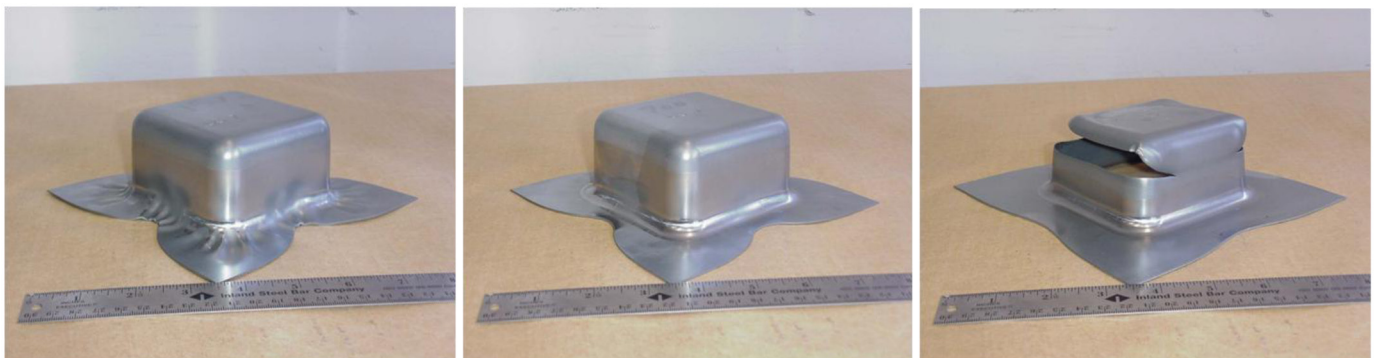
Figure 1. Effect of binder force on formability of the material
