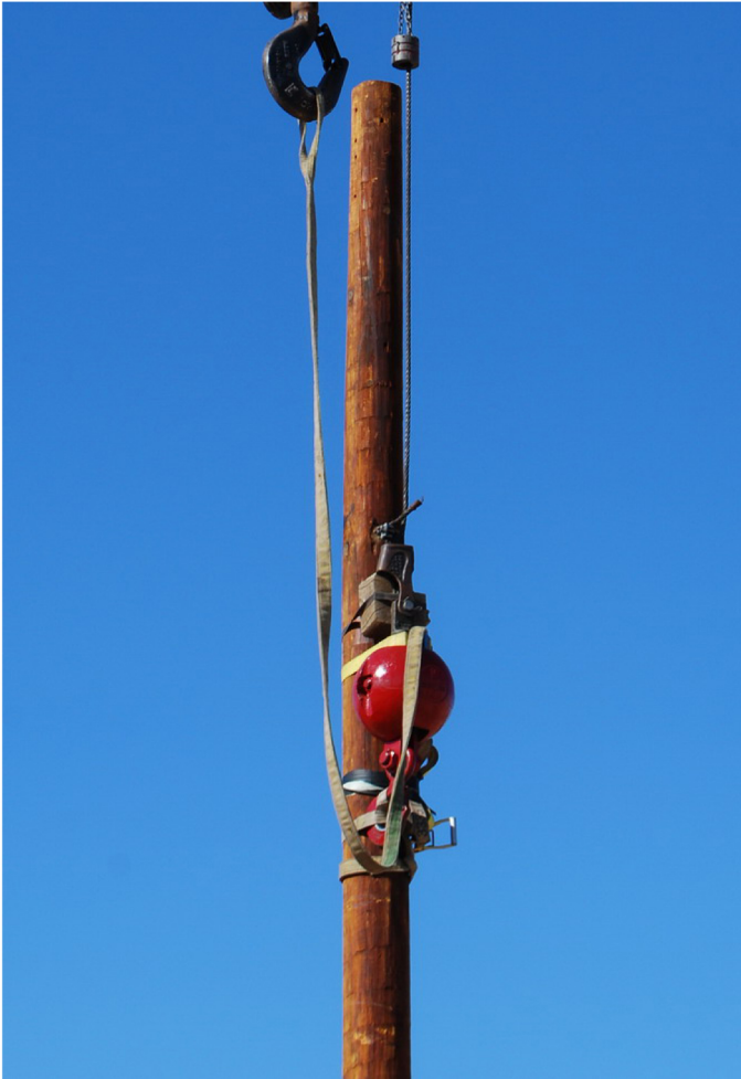
Figure 3. 400 lb spherical mass attached to pole to simulate conductor and other in-service loads.
