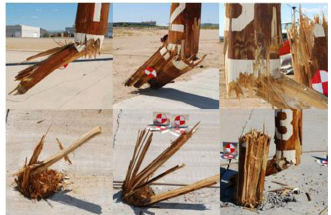
Figure 2. Brash fractures from 30 mph impact tests with a non-deformable moving barrier.
