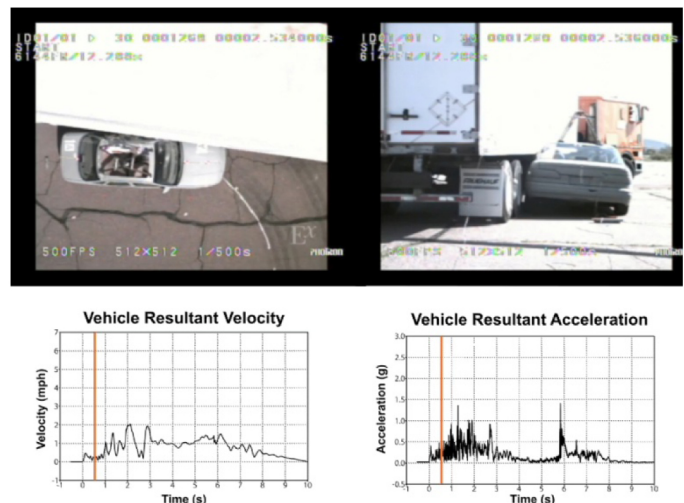
Figure 8. Test 1A: Trailer bottom rail contacts sedan A-pillar.
