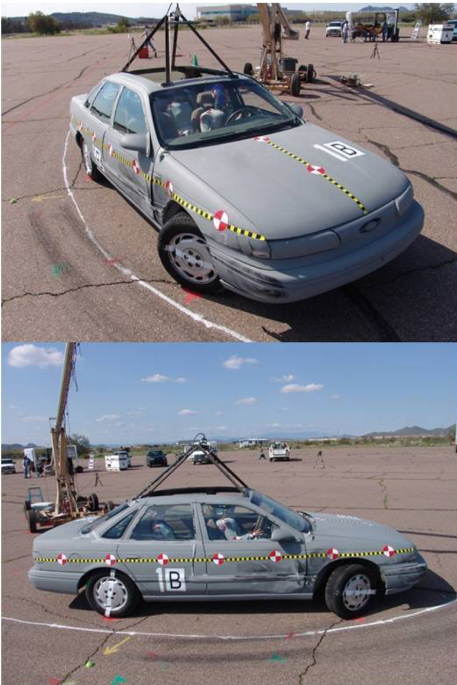
Figure 15. Test 1B post-test sedan damage
