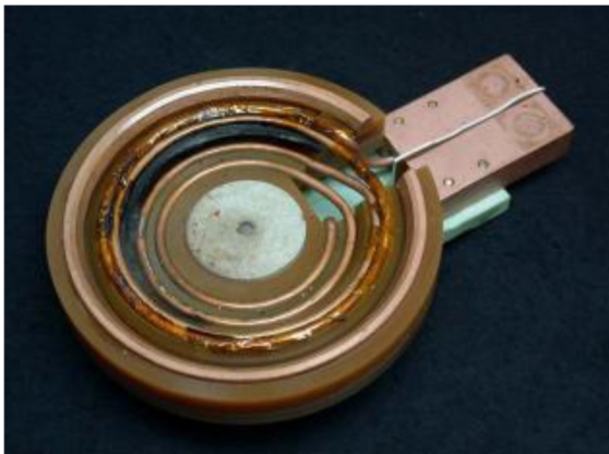
Figure 3. Induction Coil Fixture (a) and Set-up for annealing the Marciniak Test Samples (b).
