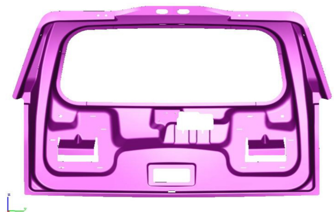
Figure 1. Liftgate inner panels stamped with (a) aluminum showing splitting fractures and (b) steel product representation.
