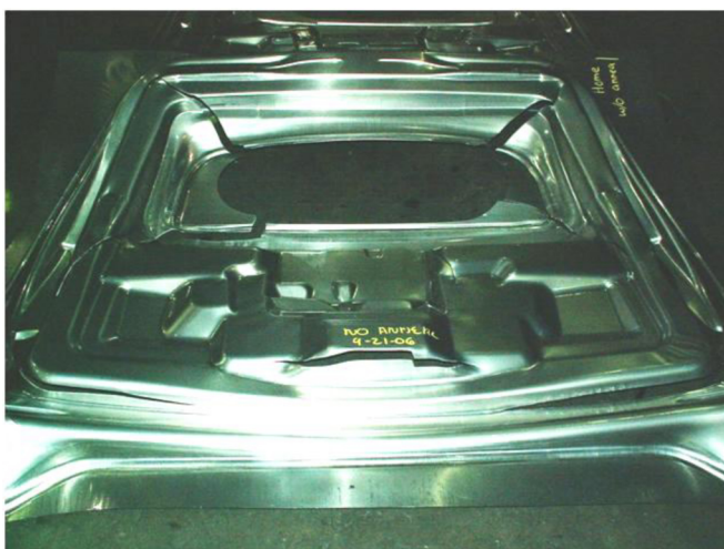
Figure 1. Liftgate inner panels stamped with (a) aluminum showing splitting fractures and (b) steel product representation.
