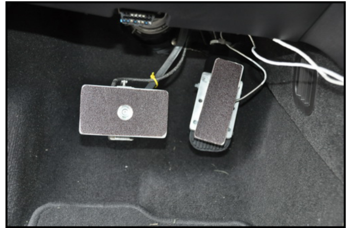
Figure 1. Accelerator and brake pedals fitted with load cells.
