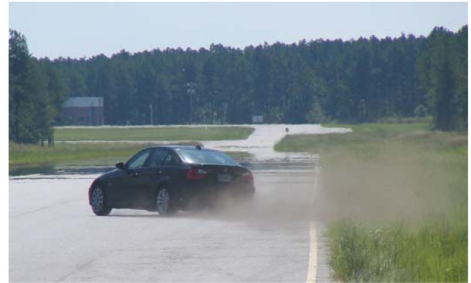
Fig. 1. Vehicle position shortly after road return during a shoulder induced event on a closed test track course
