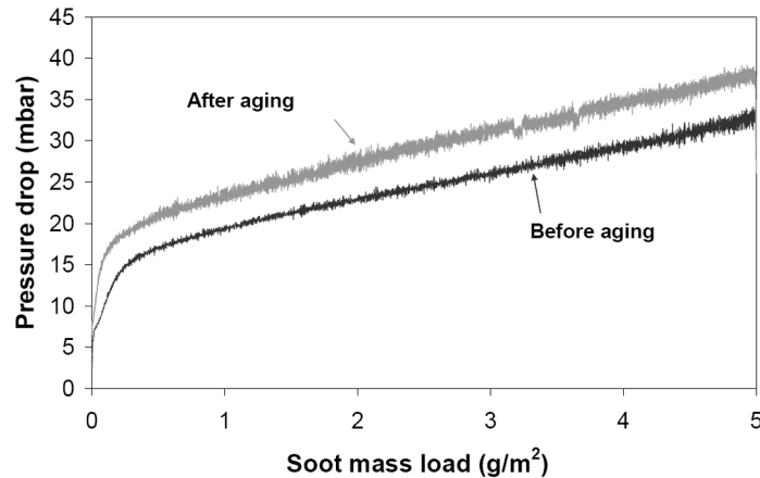
Figure 3. Evolution of pressure drop during soot loading for the fresh and the aged MFR
