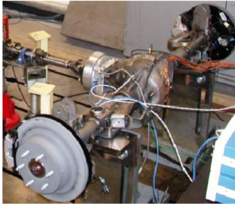
Figure 7. Stationary thermocouples on various carrier locations (C1-C15)
