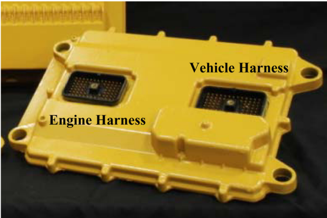
Figure 4. ADEM 2000 Engine and Vehicle Harness Locations
