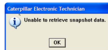
Figure 15. Caterpillar Electronic Technician Error Message Displayed When Attempting to Image Quick Stop Snapshot Data from 5EK 3406E “CA” ECMs.
