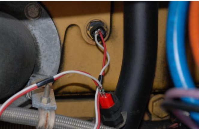
Figure 2. Interface with Intake Manifold Air Temperature Sensor.
