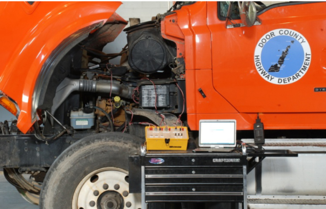
Figure 3. LEE C13 Test Vehicle with Potentiometers Hooked to Three Engine Sensors.
