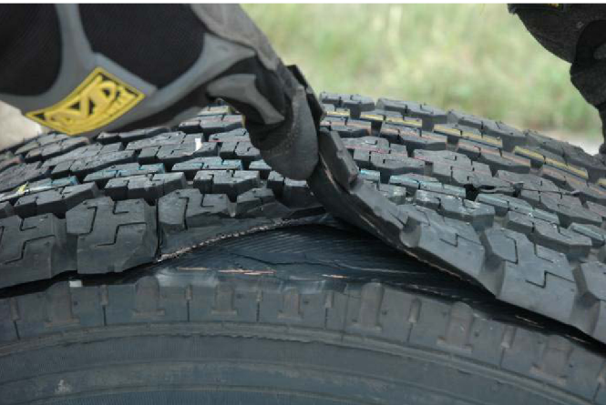
Figure 1. Test Tire Prepared to Simulate a Tread Separation
