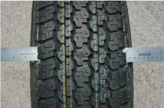
Figure 2. Test Tire Prepared to Simulate a Tread Separation
