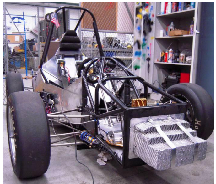
Figure 1. Front Impact Attenuator Affixed to the Front of a Formula SAE vehicle
