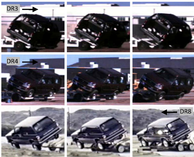
Figure 4. High speed video/film images between dolly snub and initial ground contact.
