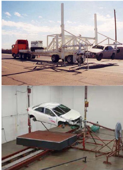
Figure 1. The CRIS test system (top) and the JRS test system (bottom). Source: Cooper et al. 2001 , and Friedman and Hutchison 2008 .
