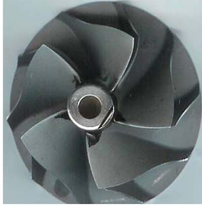
Figure 4. Actual impeller geometry (IHI RHF3 compressor) and related 3D reconstruction
