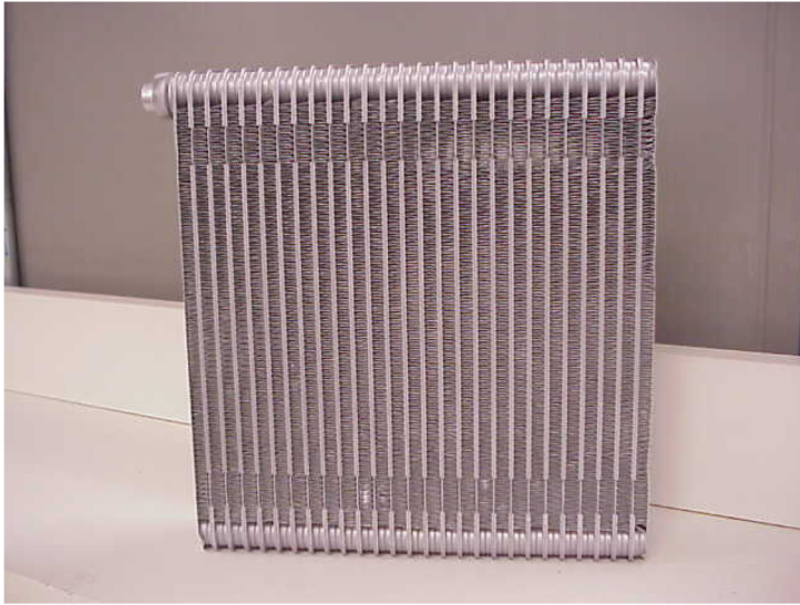
Figure 3. Photograph of the evaporator used for the current investigation
