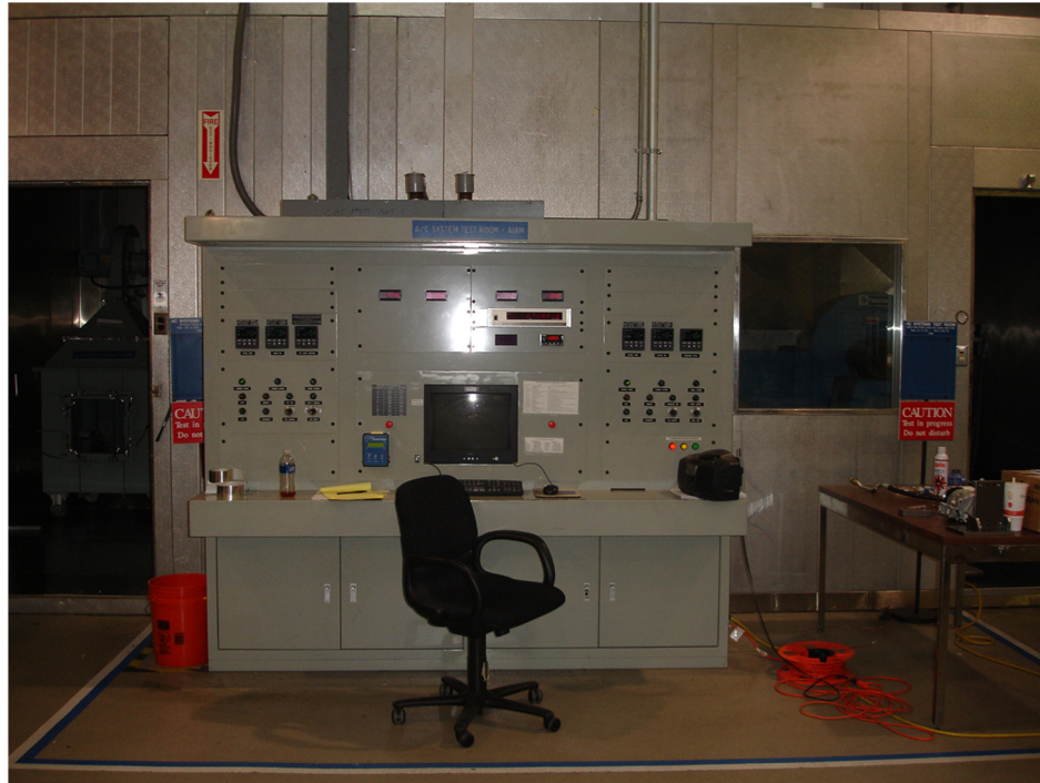
Figure 5. Photograph of the test facility - the room on the left side simulates the cabin interior; and the room on the right simulates the engine compartment.
