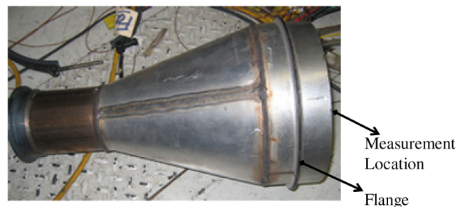
Fig. 3. Test geometry. Location of flange and measurements are also shown.
