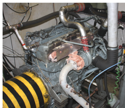
Fig. 1b. Tested engines. MAN engines used for lube oils aging at the Oil and Gas Institute, Krakow, Poland
