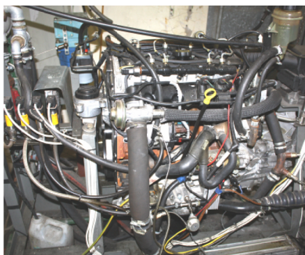
Fig. 1c. Tested engines. FORD, engines used for lube oils aging at the Oil and Gas Institute, Krakow, Poland
