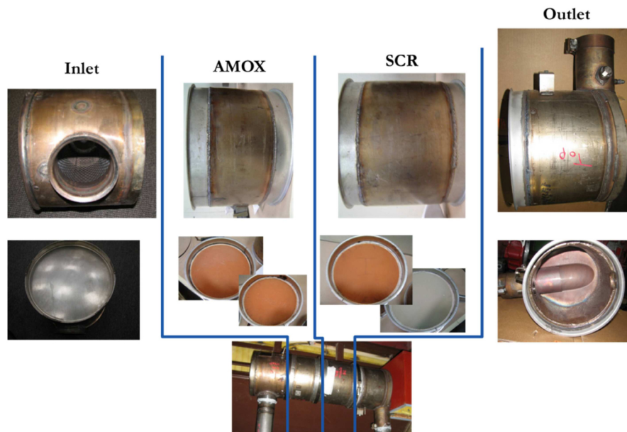
Figure 2. The SCR unit with AMOX filter, inlet and outlet end caps.
