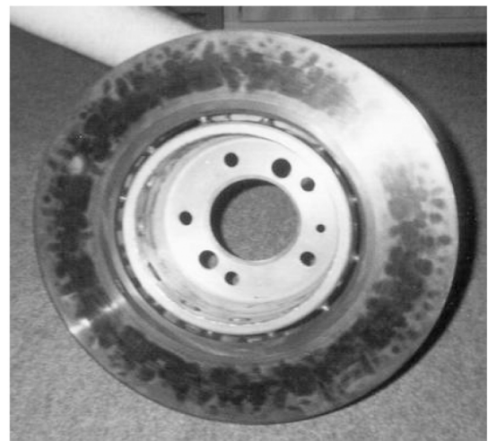
Figure 5. Extreme case of “hot spotting”. Often appears to be random but may be a function of rotor speed.
