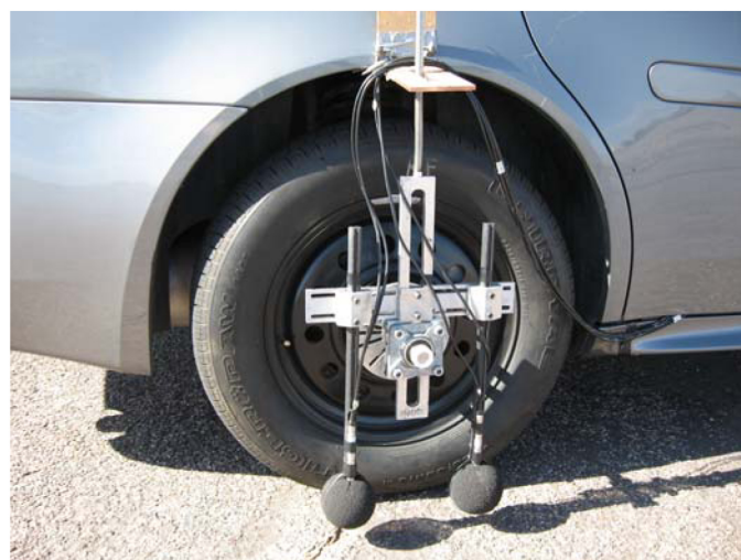
Figure 1. OBSI fixture installed on a test vehicle
