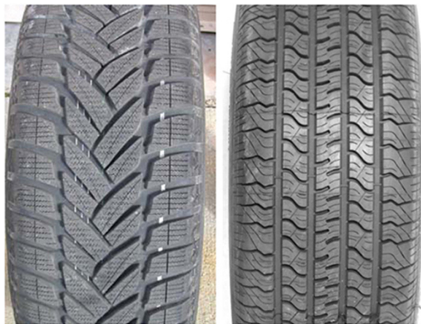
Figure 2. Test tires - Dunlop SP Winter Sport M3 on the left, ATSM Standard Reference Test Tire (SRTT) on the right
