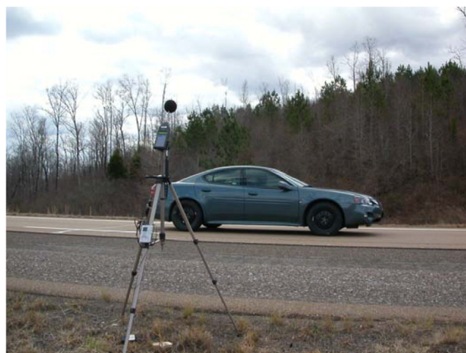
Figure 3. Pass-by measurement setup at S4
