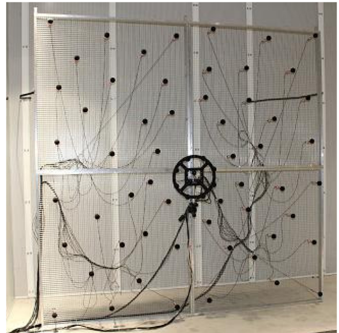
Figure 3. Grid array (3 m × 3 m) with integrated camera module.
