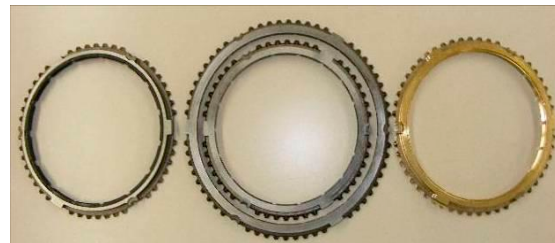
Figure 3 – Selected synchroniser rings used in this work (l-r) phenolic, carbon, molybdenum (sitting inside the carbon ring), and brass.
