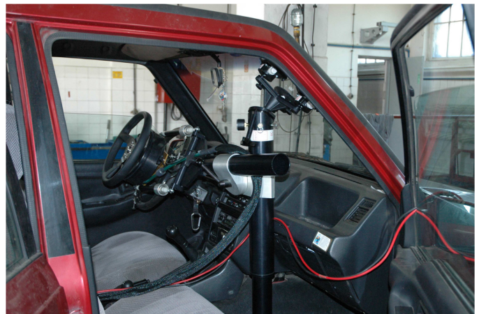
Figure 1. Installation of the steering robot in the test vehicle: a motor unit (top), a mounting fixture with torque transducers (bottom).
