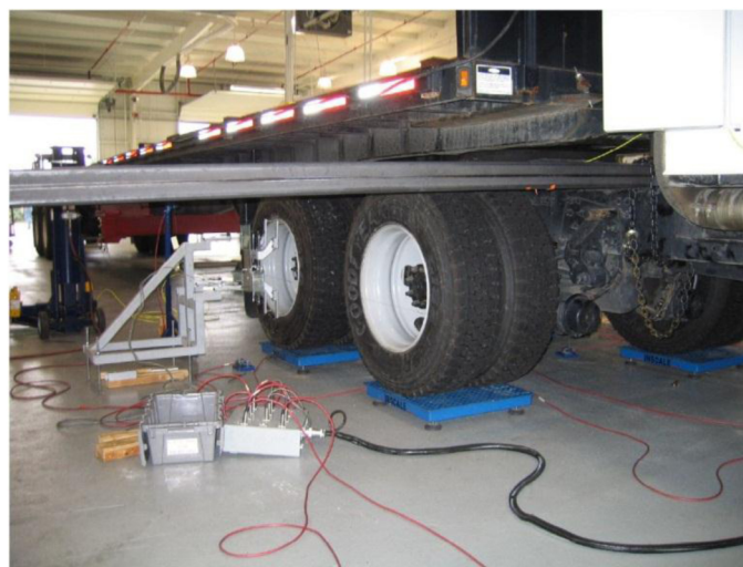
Figure 2. Torsional stiffness test apparatus.
