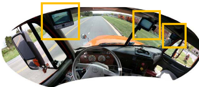
Figure 6. Placement of A-C/VIS Monitors
