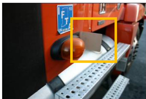
Figure 7. Translucent Plastic Light Diffusers Mounted in Front of Optional Side Turn Signal Lights
