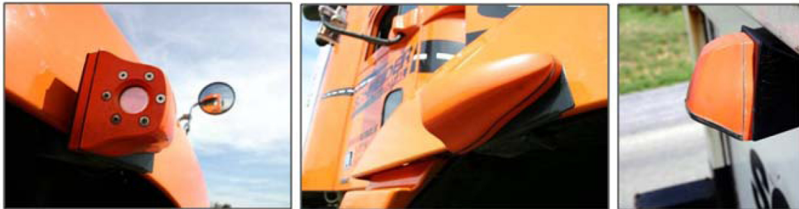
Figure 4. A-C/VIS Cameras Mounted on Truck Exterior
