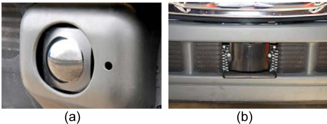
Figure 2. Some of the FCMS that are available on the market include the Bendix Wingman System (a) [2] and the Wabco OnGuard System (b) [3]. Typically these systems are mounted on the front bumper of the commercial vehicle.
