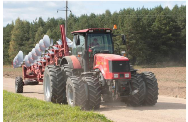
Fig. 3. Prototype tractor with EMD
