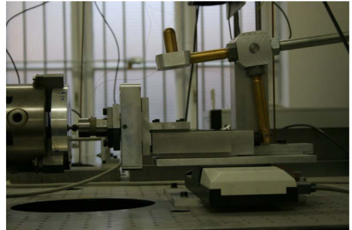
Figure 2. Experimental setup of the pin-on-disc tribometer.
