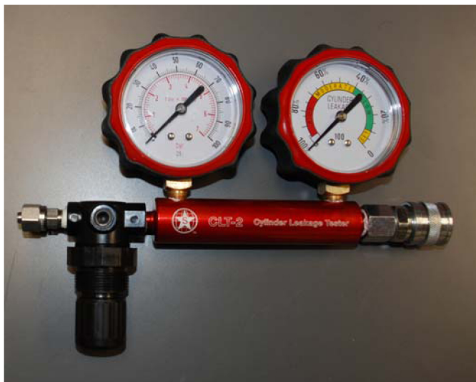
Figure 2. Photograph of a Star Products Model CLT-2PB Cylinder Leakage Tester.
