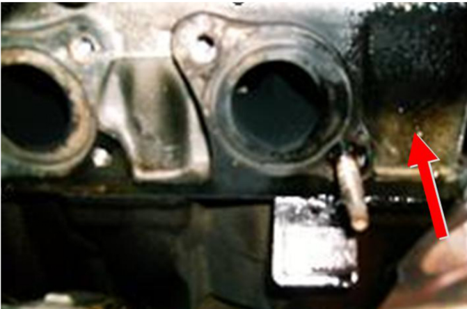
Figure 2. Gasket leakage around port IV, which is closest to turbo outlet
