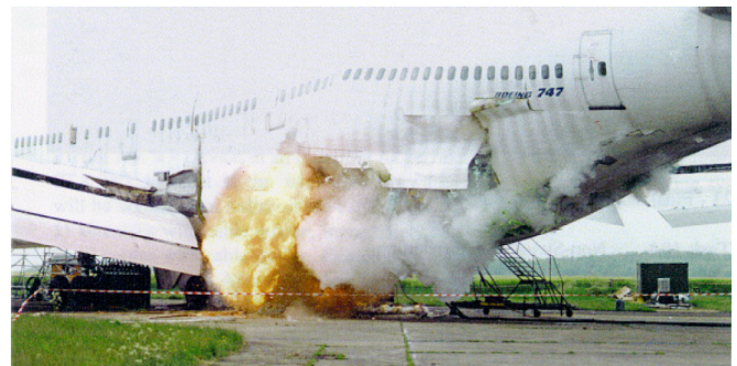
Figure 2. Destruction of wide-body aircraft by internal explosion (from [3]).
